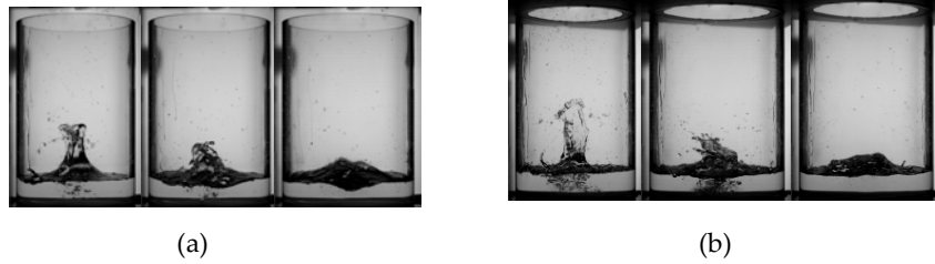
Figure 9: Decay of sloshing motion in exp3. (a), water, (b), alcohol. The images are taken at 400 ms interval
