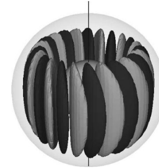
Fig. 3: Convection columns in a rotating spherical fluid shell for \tau = 10^4 , R = 3.8 \times 10^5 , P = 1 . Dark and light surfaces correspond to a constant positive and negative value of the radial velocity.
