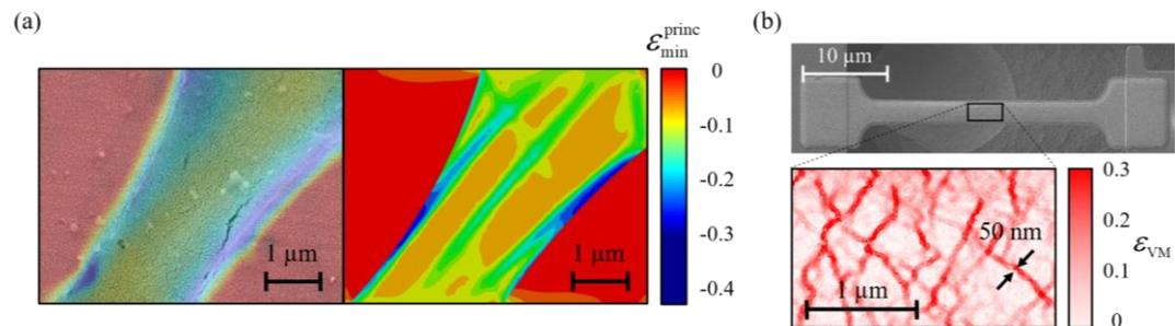
Fig. 1: (a) Minimum principal strains  $\epsilon_{\min}^{\text{princ}}$  obtained by DIC (left) and FEM (right) in a methacrylic composite under compression, and (b) Von Mises strain  $\epsilon_{\text{VM}}$  obtained by DIC in an aluminium thin film under tension
